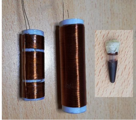
Figure 7. The coil system consisting of transmitter/driver and gradiometer receiver coil.
