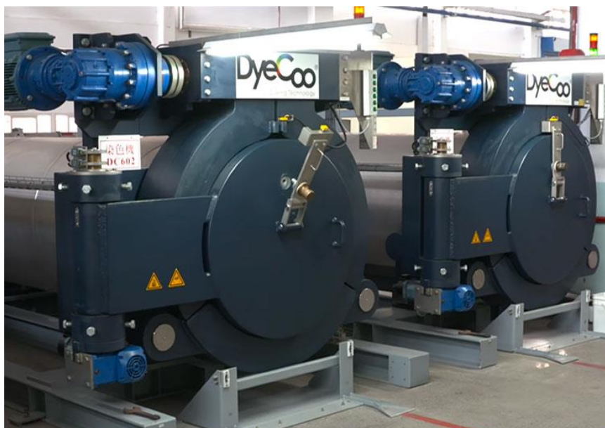
Figure 3. Commercial scale DyeCoo brand supercritical carbon dioxide dyeing machine ( https://www.ecotextile.com )
