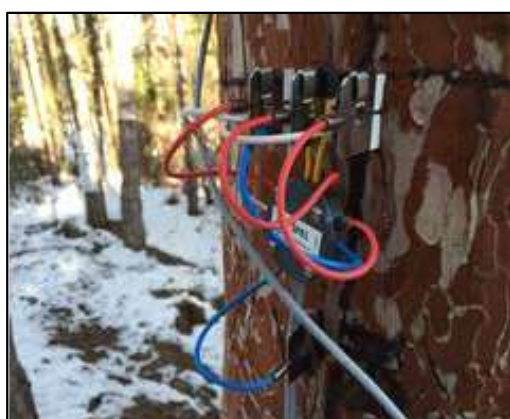
Figure 2: EMS 81 Sap flow system with electrodes and thermosensors on a tree trunk
