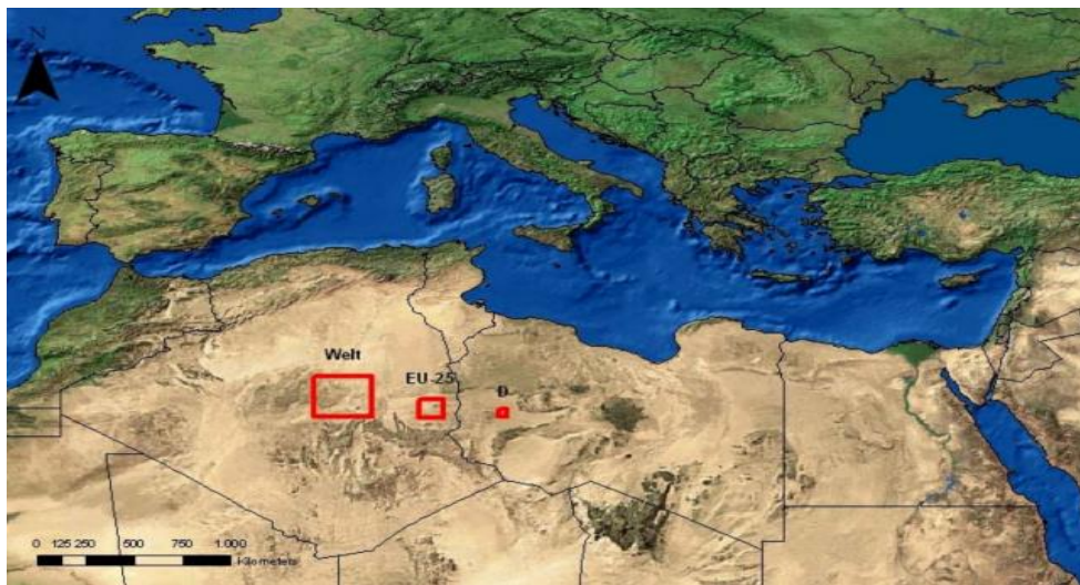
Fig. 2: Theoretical space requirement to meet the electricity demand of the world, Europe (EU-25) and Germany (May, 2005)
