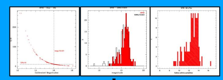
New instruments allow us to reach up to 16th magnitudes, without filter, with the 40 cm and roughly 13th magnitude with the 8 cm telescope.
