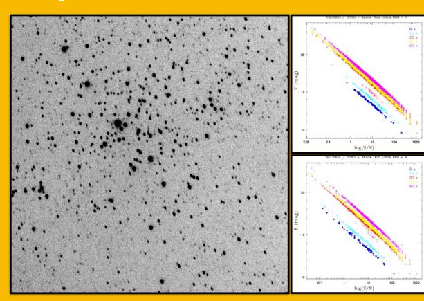
A V band image of Galactic open cluster NGC 6834 obtained with ANDOR iXon Ultra 888 EMCCD with a 30s exposure time. The panels to the right show the reached signal to noise ratio for a range of magnitudes as a function of different exposure times.
